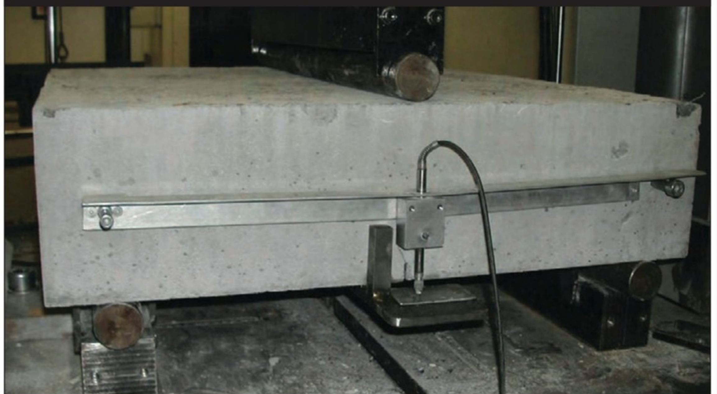
Figure 3: Three point bending test on square panel with notch (from de Rivaz)
