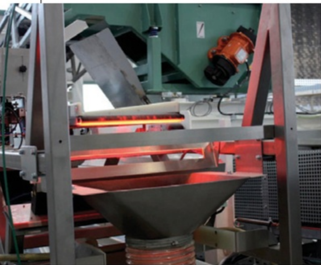
Above: Photo-optical system for in-line characterisation of spoil - laboratory prototype for the DRAGON project (Galler, 2015)
