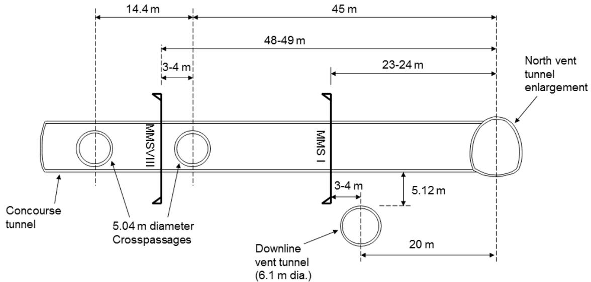
Figure 2: Long section of the Concourse Tunnel showing locations of MMS I and MMS VIII
