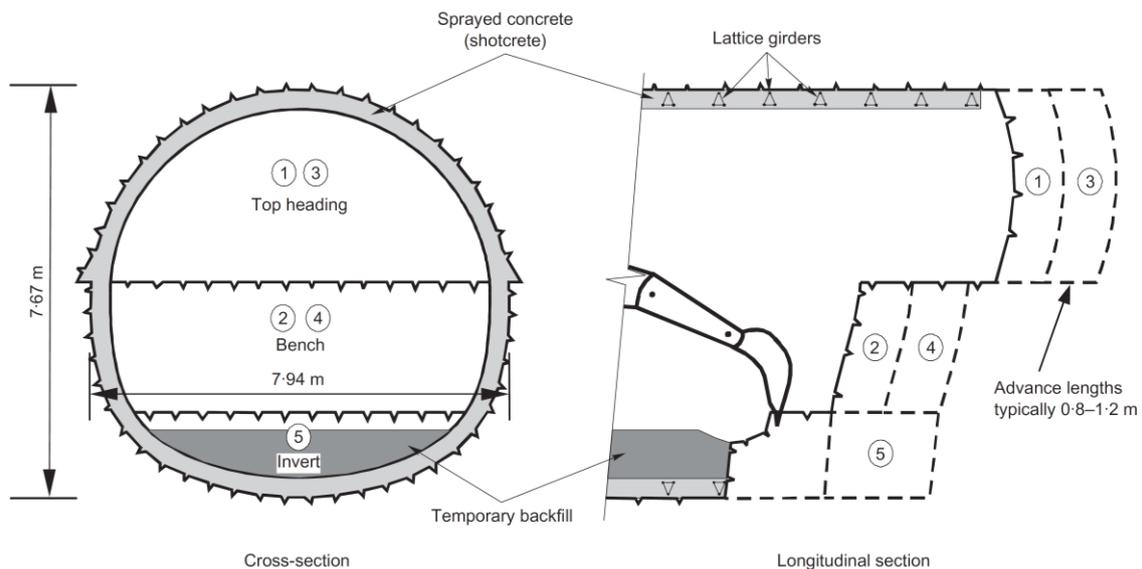
Figure 1: Concourse Tunnel construction sequence (from van der Berg et al., 2003)
