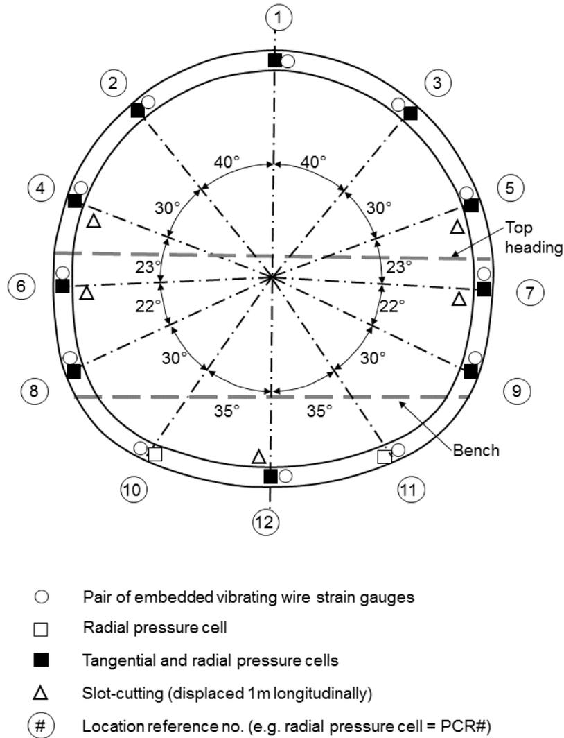
Figure 3: Main monitoring section schematically showing locations of pressure cells and strain gauges embedded in the sprayed concrete primary lining
