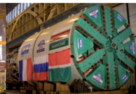
Soft ground TBM
