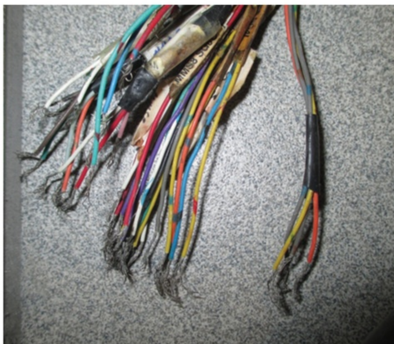
Figure 3 (left): One of several multicore cables required for 2 arrays of instrumentation (pressure cells and strain gauges) installed at Heathrow Terminal 4 station in 1996 (photo taken in 2015)
