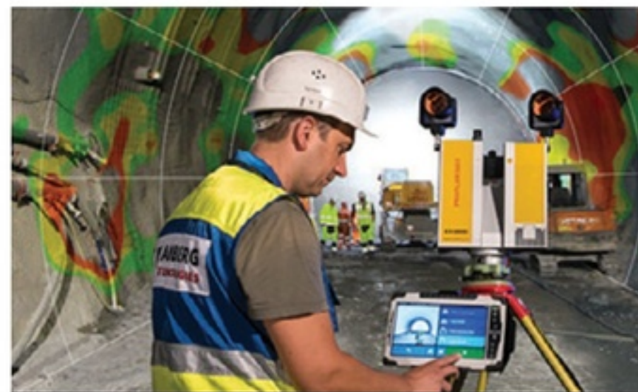
Figure 1 (above): A stationary laser scanner for tunnel profile measurement (www.ambergtechnologies.ch)
