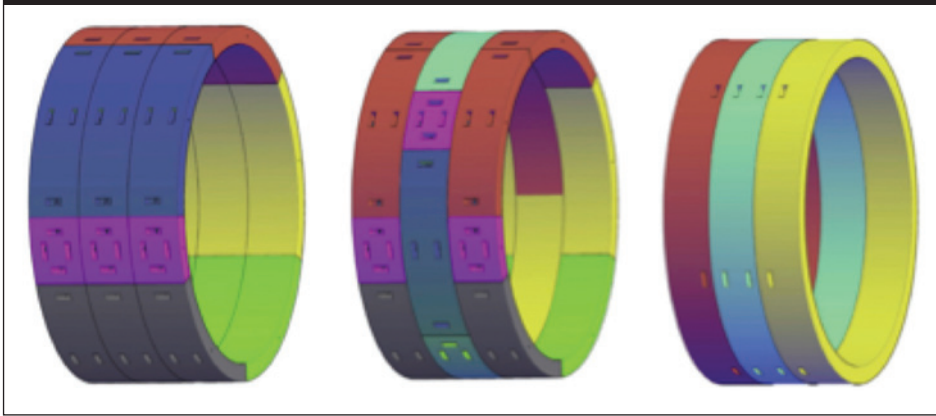
Figure 3: Effect of ignoring circumferential joint shear resistance ('uncoupled', left) and modelling circumferential joint shear resistance ('coupled', right) (from Klappers et al., 2006)
