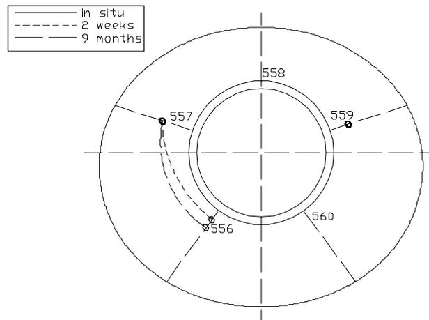
Fig. 12: Radial pressures at T5 Array 2 at 2 weeks and 9 months
