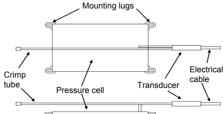
Fig. 1: Geokon 4850 series pressure cells
