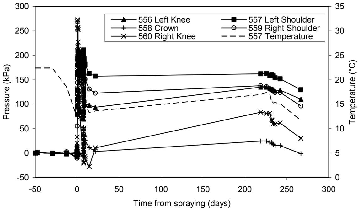
Fig. 4: Recorded pressures in T5 array 2 radial cells
