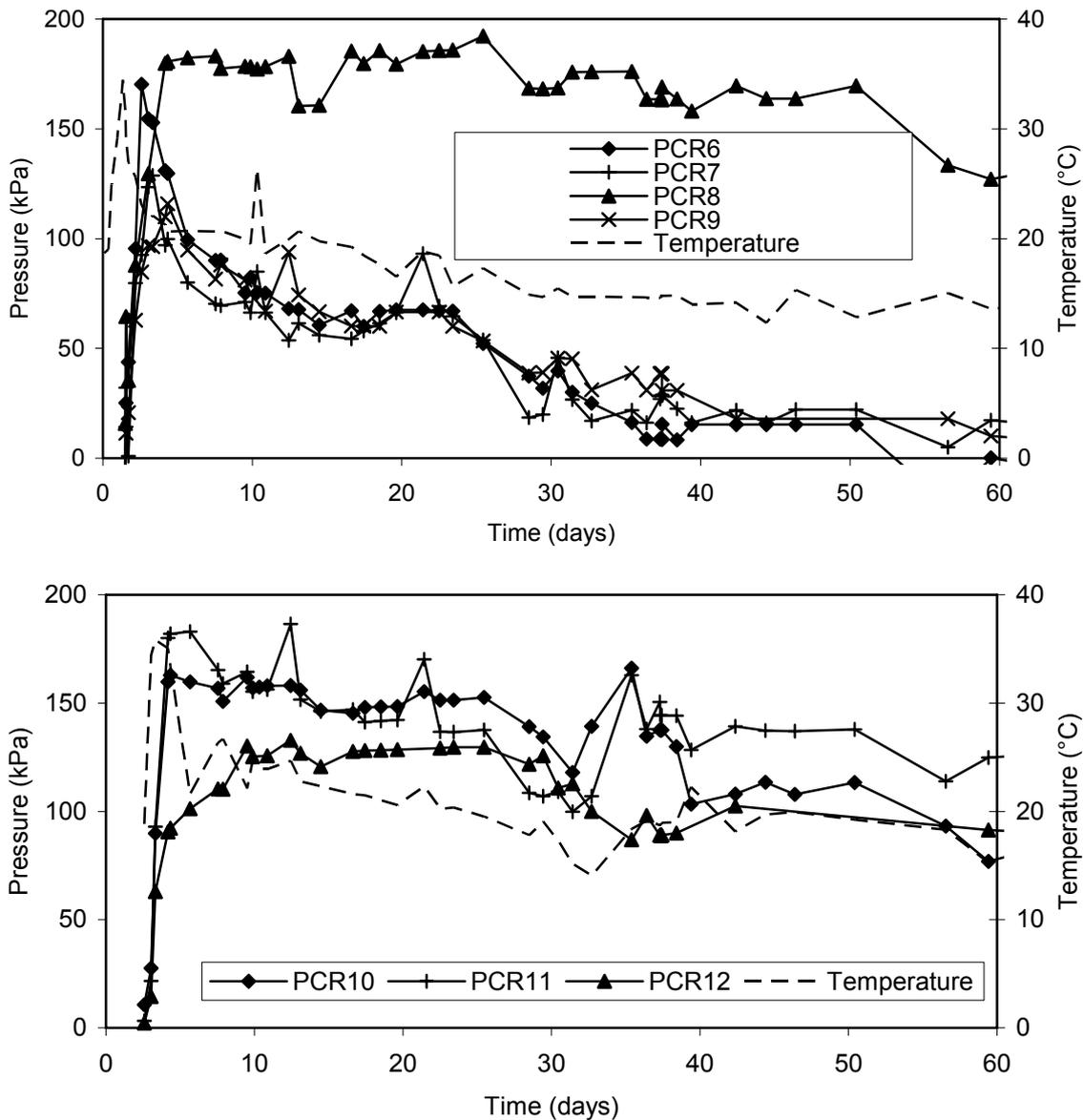
Fig. 7: Recorded pressures on the (a) top heading, (b) bench, and (c) invert at MMSI, T4
