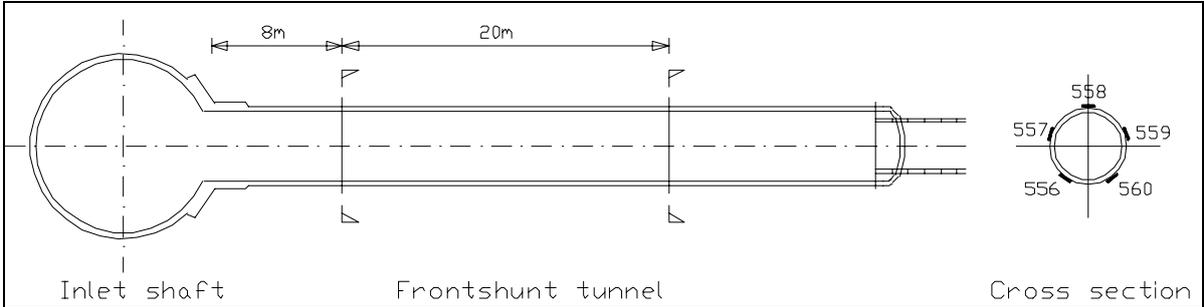
Fig. 2: Plan and cross-section of T5 pressure cell locations.
