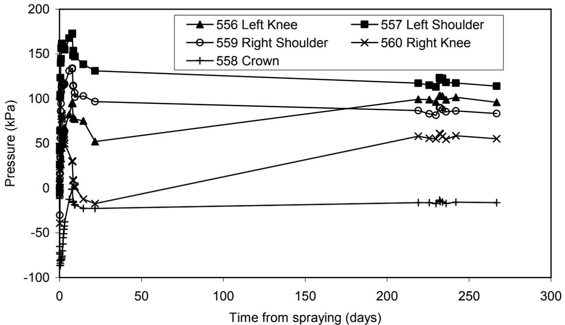
Fig. 5: Adjusted pressures in T5 array 2 radial cells.
