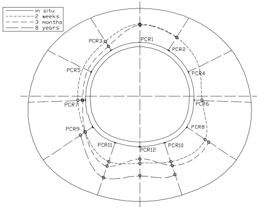
*Fig. 10: Radial pressures at MMSI at 2 weeks, 3 months and 8 years*
