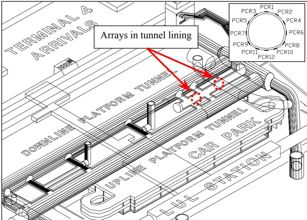
Fig. 6: Isometric view and cross-section of Terminal 4 Station pressure cell locations
