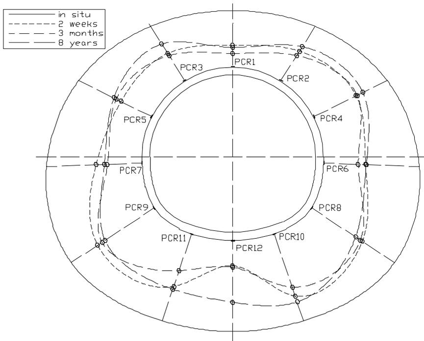
*Fig. 11: Radial pressures at MMSVIII at 2 weeks, 3 months and 8 years*
