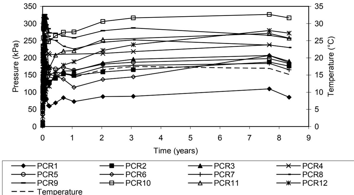
Fig. 9: 8 years of recorded pressures at T4 MMSVIII
