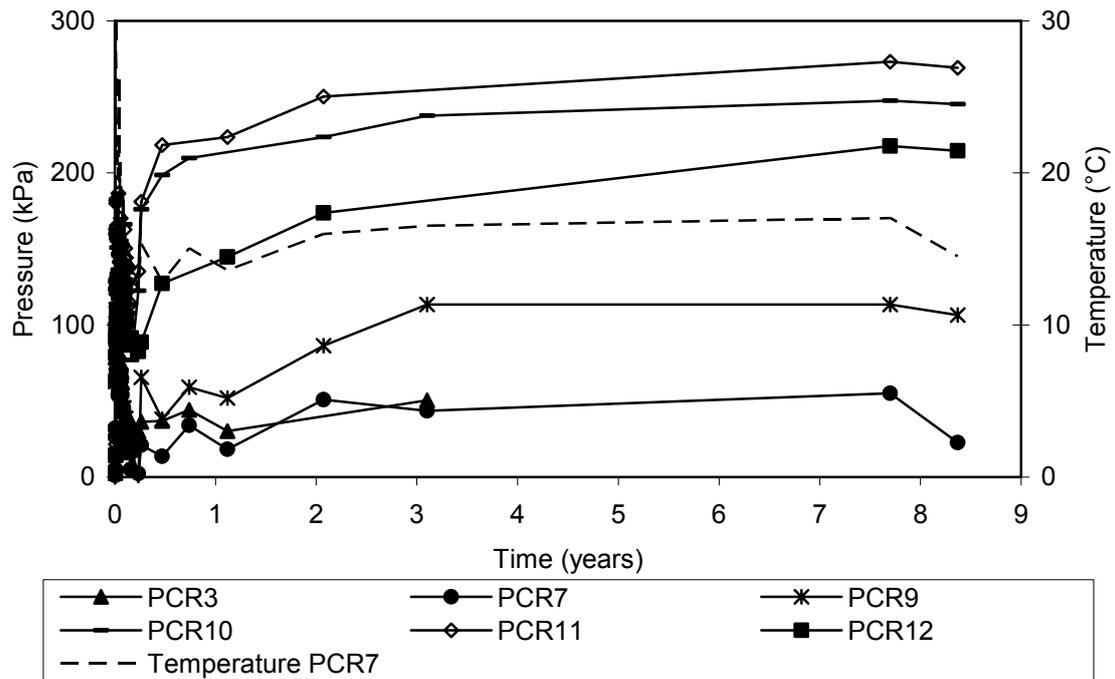
Fig. 8: 8 years of recorded pressures at T4 MMSI
